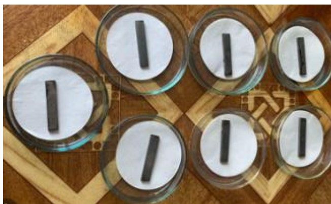
Figure 2. Samples of 17GS steel after exposure in a model environment with the addition of various green corrosion inhibitors - preparation for mass loss analysis.
