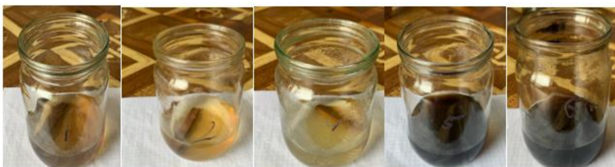
Figure 1. Visual comparison of steel samples after exposure to the NS4 model environment with the addition of various plant corrosion inhibitors.
