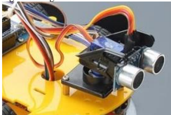
Fig. 19. Rangefinder, stationary fixed on top platform chassis.
