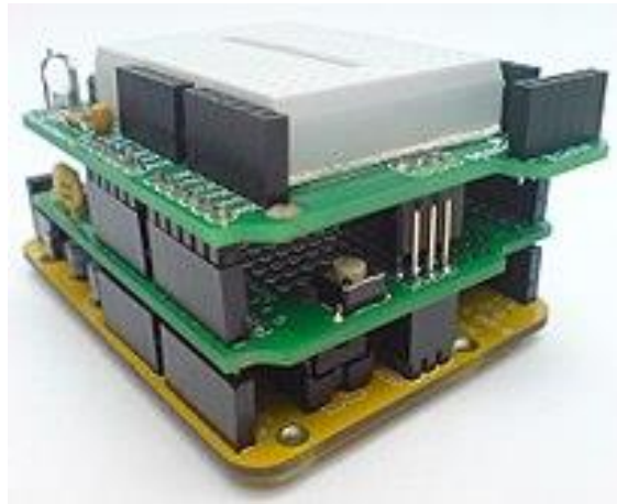
Fig. 1. Standard Arduino design with boards extensions.
