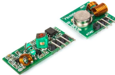
Fig. 3. Set radio modules: transmitter FS 1000A and receiver MXR 5V.
